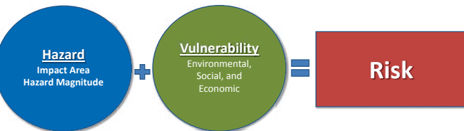
Fig. 1. Factors involved in determining natural hazard risk
